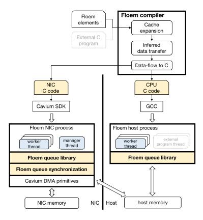
Figure 3.4: Floem system architecture
