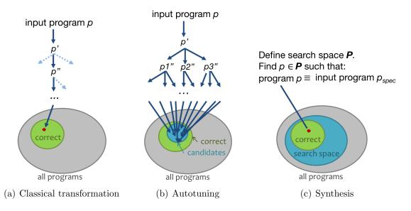
Figure 1.1: Comparison of different compilation techniques
