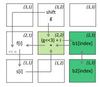
(c) Layout and routing. Partition xy is mapped to physical core (x, y). Dark and light green denote actor cores of  $\mathtt{get\_b}$  and  $\mathtt{step}$  respectively.
