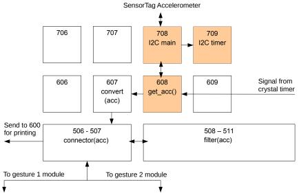
(a) Program layout of accelerometer reading and data filtering
